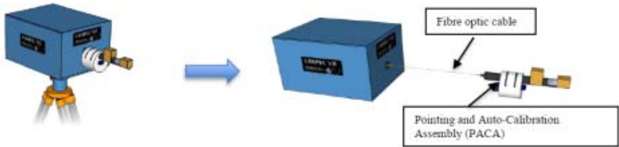
図2. Simple reconfiguration for fast airborne and vehicular surveys
